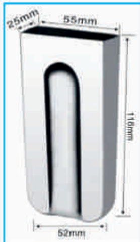
ICE-1053 ICE CREAM MOLD CAPACITY MAX =116ml FILL LINE 6mm =109ml FILL LINE 20mm =118ml
