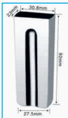
ICE-1057 ICE CREAM MOLD CAPACITY MAX =60ml FILL LINE 6mm =55ml FILL LINE 20mm =47ml
